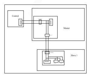
Unique series-connection , could connect two SB steam generator (Up to 18KW) to output 24KW-36KW large steam generator, and use only the same one control panel to avoid the high cost of using large commercial steam generator.
